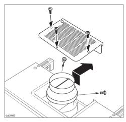
For Recirculation the reducing collar with the non-return flap must be removed by unscrewing the screws and installing the recirculation grille.
